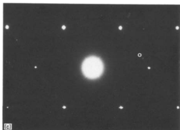
Figure 3 Thick twins in the sodium-modified dendrite shown in Fig. 2a. (a) Bright-field image. (b) Centred dark-field image using the marked twin spot in Fig. 3c. Thin twins are visible as well as the thick twins because the objective aperture covered part of the \langle 111 \rangle streak. (c) \langle 110 \rangle diffraction pattern: Fig. 3b was formed using the marked faint spot. (Image-pattern rotation has not been corrected).
