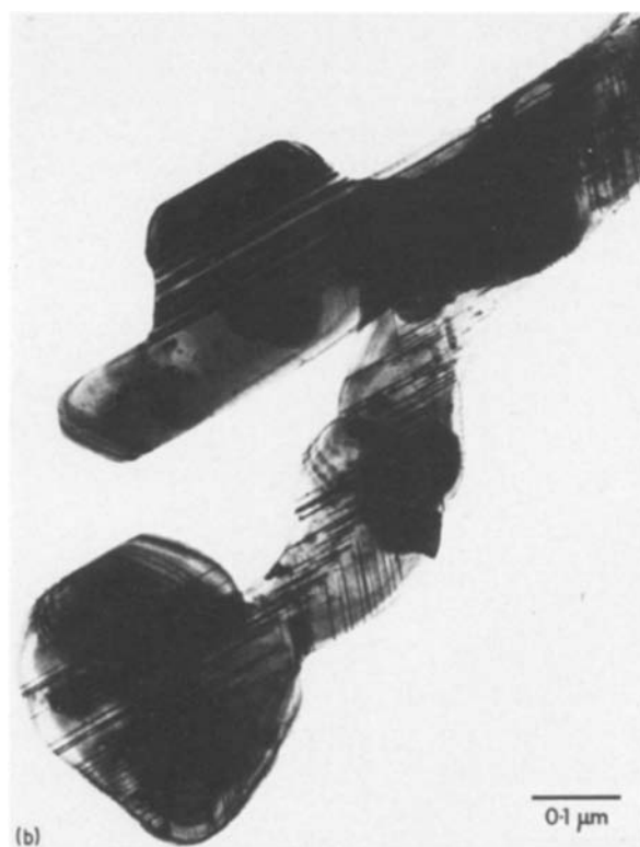
Figure 4 Thin \{111\} fault distribution in modified silicon; \langle 110 \rangle zone axis. (a) Quench-modified Alloy Q. (b) Strontium-modified Alloy D-Sr.
